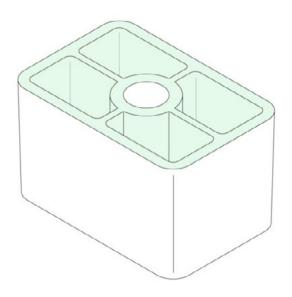
Reducing the wall thickness of your part is the best way to minimize the part volume. This way not only less material is used, but also the injection molding cycle is greatly accelerated.
