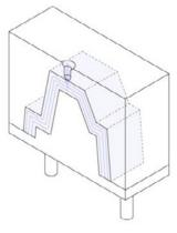
This is a fundamentally different way of manufacturing compared to additive (3D printing) or subtractive (CNC machining) technologies. The flow and solidification of the material during injection have a significant impact on the key design restrictions for this technology - more on this in below.
