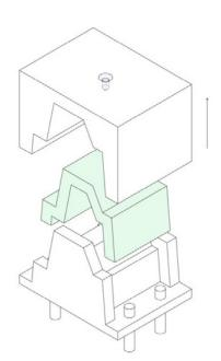
Side-action cores and the other in-mold mechanisms can increase the cost of tooling by 15% to 30%. This translates to a minimum additional cost for tooling of approximately \$1,000 to \$1,500.
