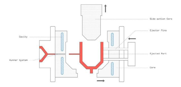
The simplest mold - the straight-pull mold - consists of two halves: the cavity and the core. For more complex parts with 'undercuts, side-action cores can also be used that slide in and out of the part on an angle - more on side-action cores & undercuts in a next section.
